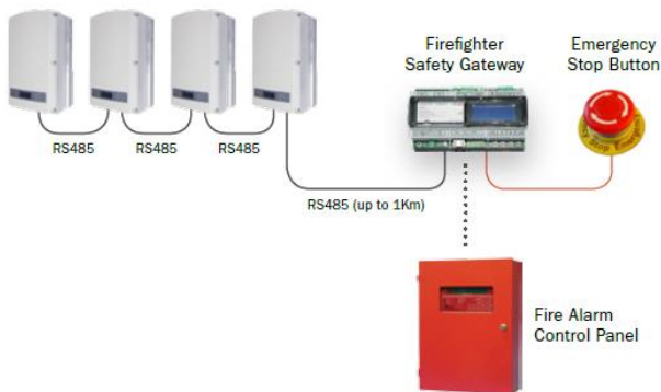
Figure 2: The SolarEdge Firefighter Gateway Connections
