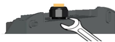
Fig. 6-15: Tighten the cable gland from the back
