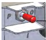
ON/OFF/P Switch: 0 = OFF 1 = ON P = Pairing
